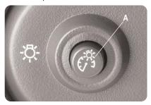
If the interior lamps are left on for more than 10 minutes with the ignition off, the Battery Rundown feature turns them off.
